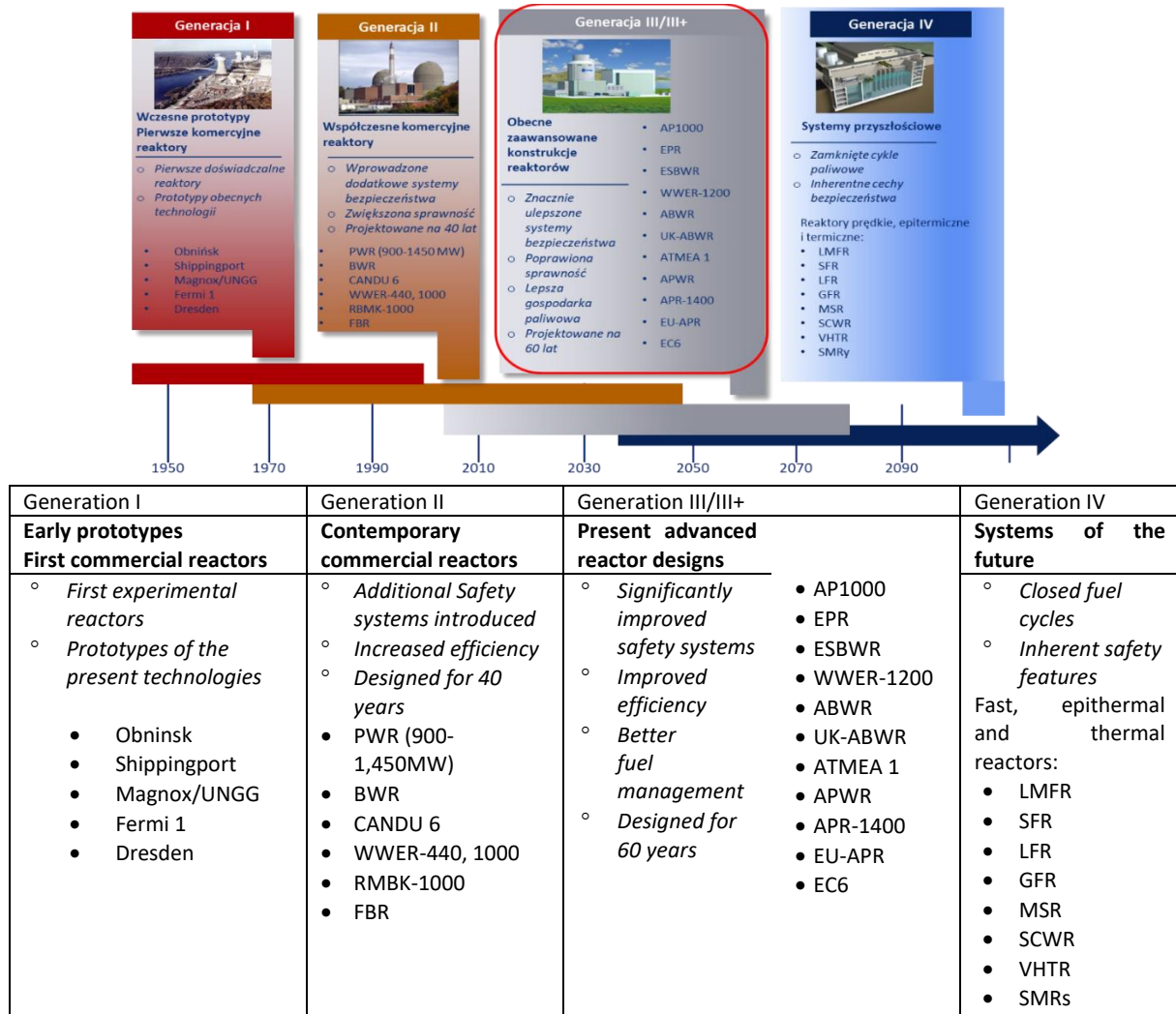
Figure I.- 2 Generations of nuclear power plants
