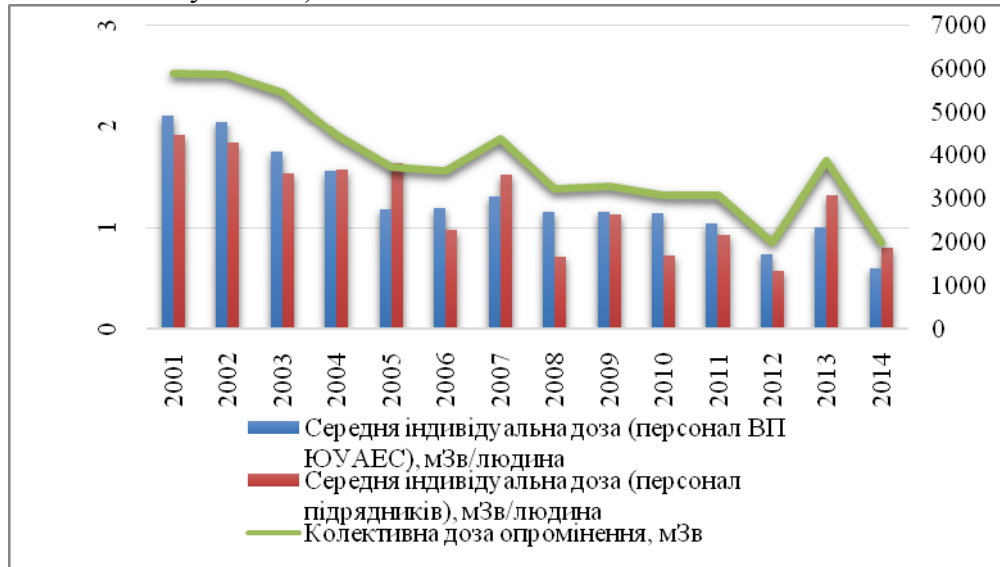
Fig. 3.6. – Dynamics of individual and collective annual doses of accumulated exposure (external and internal one) at SUNPP
