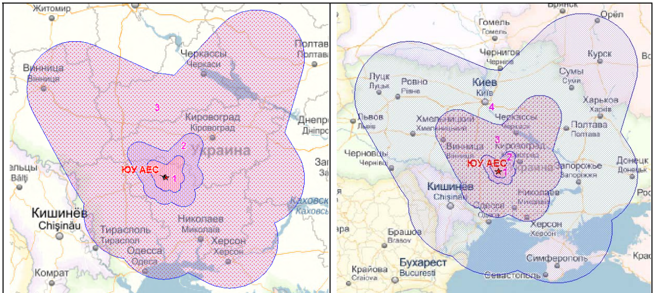
Fig. 6.7. – Probable activity of tritium radionuclides fall outs on the ground due to the transfer of atmospheric emissions of SUNPP.
