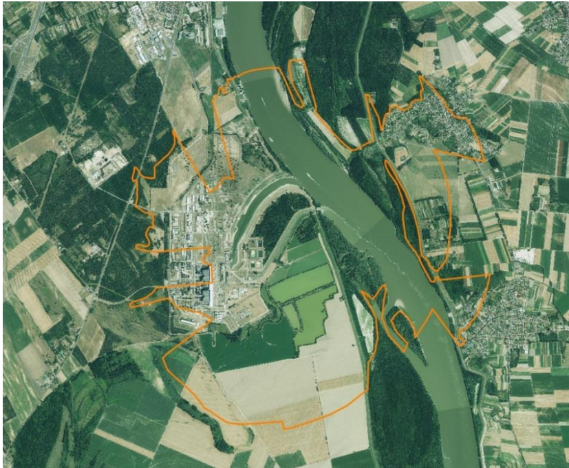
Figure 3.4-7: Noise exposure impact area of the joint operation of Paks II. and Paks Nuclear Power Plant
