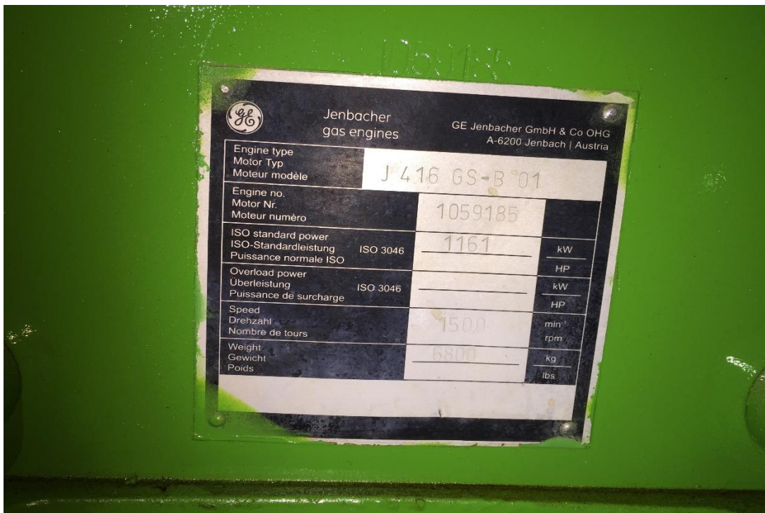
Image 3: Gas engine nameplate
