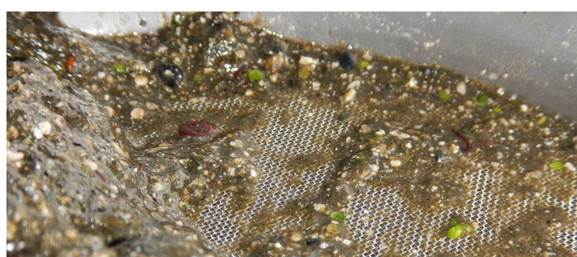
Fig. 1: Solid residues of clean WWTP-effluent (waste water treatment plant), separated on-site from 500 m 3 of WWTP-effluent by 250 µm mesh net.
